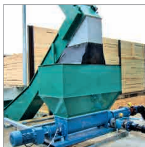
Feeding the pump via a transferring hopper
