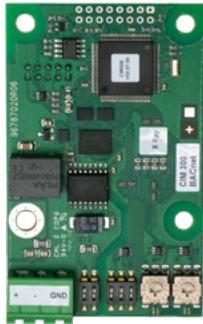
Biral Interface Module for communication via a BACnet MS/TP network
