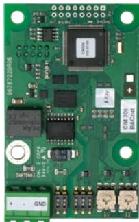
Biral Interface Module for communication via a Modbus RTU network
